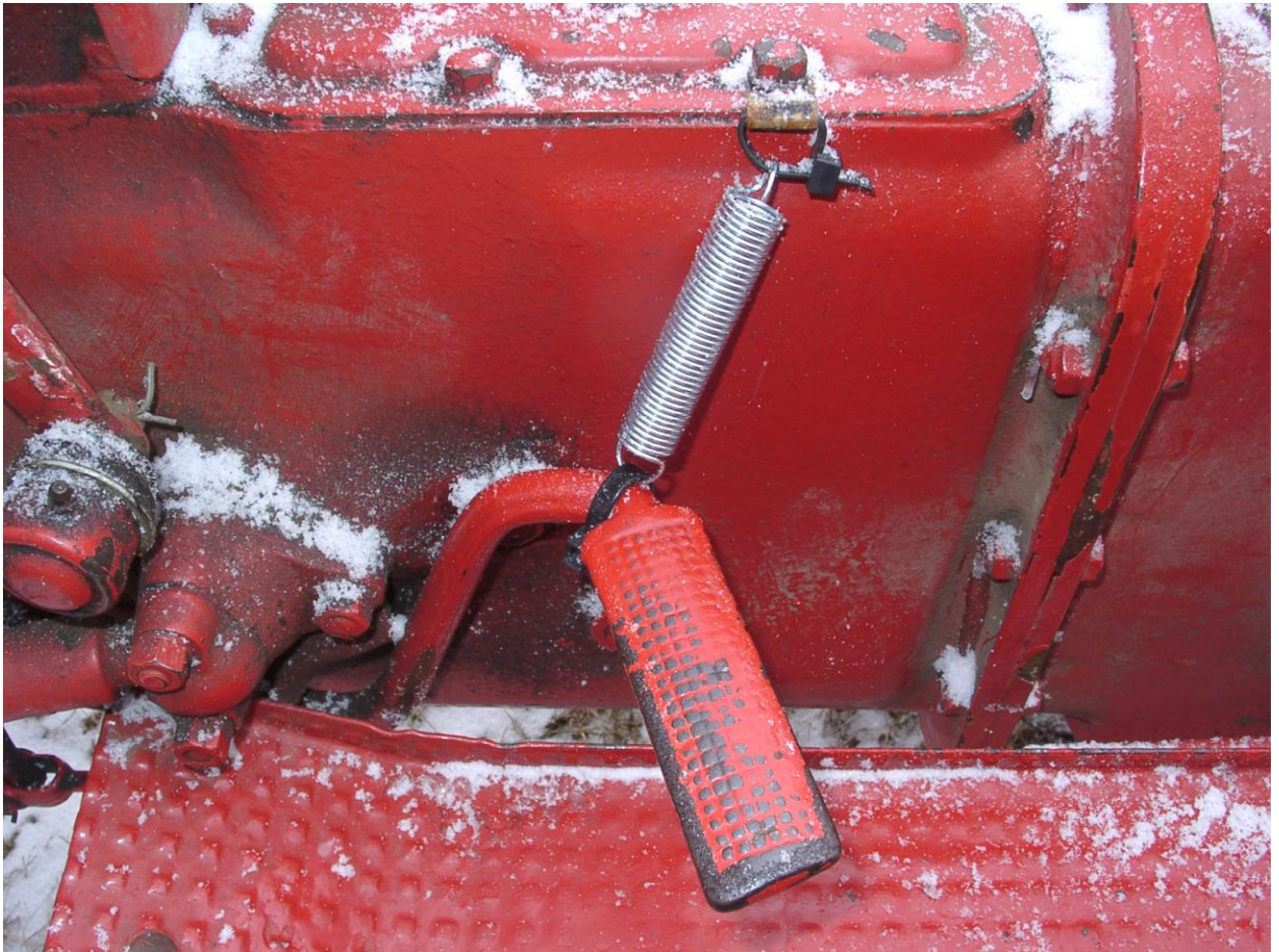
FIG 6 –Test drive the tractor and adjust spring tension as needed. After the spring stretches out a bit, you may need to readjust tension again.
