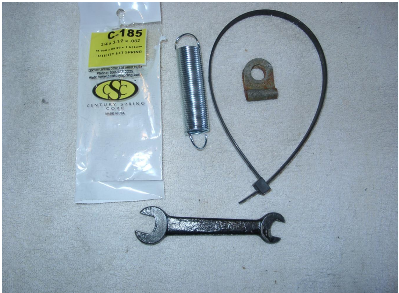
FIG 2 –Parts List –one 3-1/2” HD spring; two HD wire ties; and one lamp wiring clip. You’ll also need a 5/8” wrench and a pair of wire cutters.
